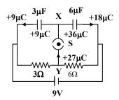
Initial charge distribution (when switch S is open)
