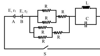
**Sol.** Since average voltage across capacitor and inductor for D.C. sources will be zero at steady state.
